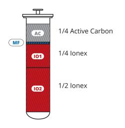
We can combine the cartridges, even in one housing. Final composition of cartridges is set according to cleaning application.
