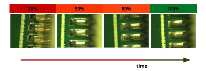
All conclusions are based on **visual inspection** under microscope and **ionic contamination testing** before and after cleaning.
